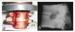
Fig. 5. Thoracic FSU's with simulated microdiscectomy. a – before testing, mounted in Electro Mechanical Testing Machine, Zwick 1464 (Germany); b – radiograph after load increment.
