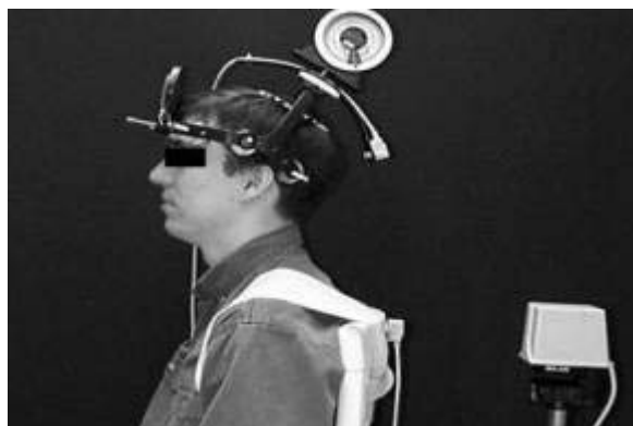
Figure 2. Subject performing cervical spine flexion maneuver while wearing the cervical spine measurement apparatus. Note the subjects' torso is restrained, to reduce torso move-
