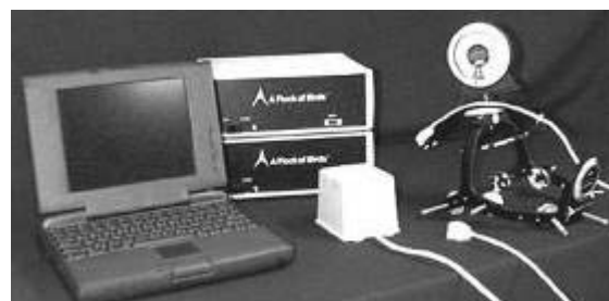
Figure 1. Spinal Kinematic assessment system, consisting of (magnetic tracking system transmitter, receivers, and control units), laptop computer, and modified halo apparatus with magnetic receiver
