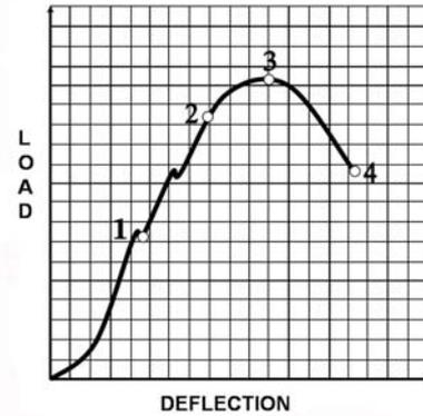
Fig. 6. Schematic load deflection curve illustrating alterations in FSU during compressive load. 1 - end plate fractures; 2 - proportional limit; 3 - yield point; 4 - total failure.
