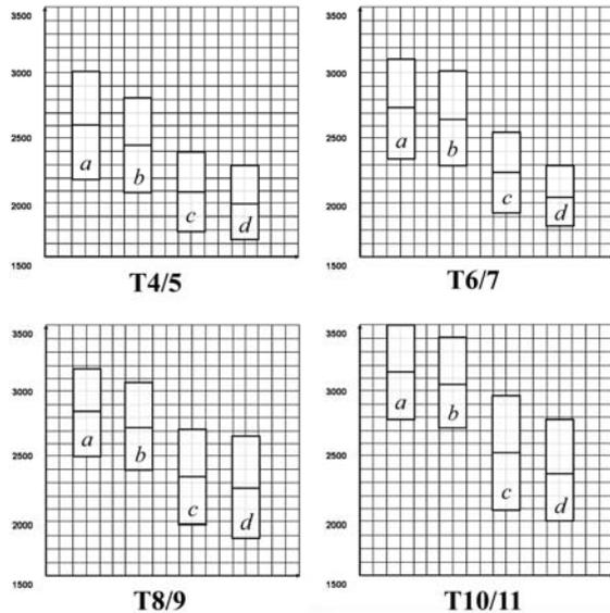
Fig. 7. Thoracic FSU's strength characteristics at the proportional limit. a – intact state under axial load; b – intact state under flexion load; c – after discectomy under axial load; d – after discectomy under flexion load. Bars show the low, average and high values for the specimens
