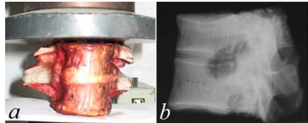
Fig. 5. Thoracic FSU's with simulated microdiscectomy. a – before testing, mounted in Electro Mechanical Testing Machine, Zwick 1464 (Germany); b – radiograph after load increment.
